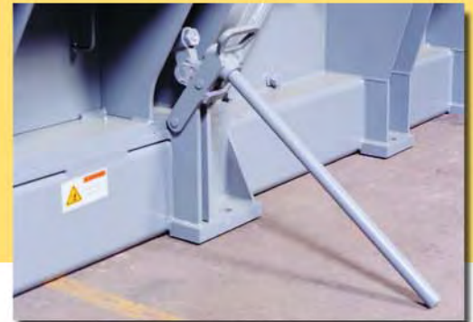
Two-piece housing is secured by simple toggle clamps, retractable pedestal by compound toggle clamps, as shown. Stedman-furnished, removable handle actuates both types of clamps. When not in use, handle is stored conveniently in base of mill.
