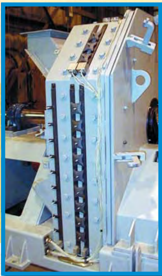
Heaters (shown with guards removed) are installed on the "H" Mill housing to retard build-up of wet material.
